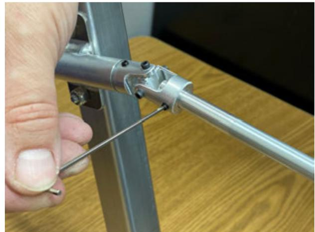
Use the 5/64" hex wrench on the set screw to remove the wand handle from the articulated joint. This will make it much easier to lower the end of the articulated joint through the opening in the ceiling tile.
